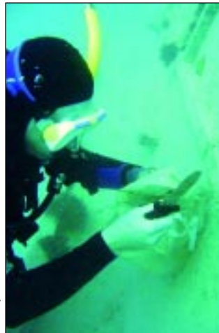
Samples are scraped from underwater structures during port surveys.
