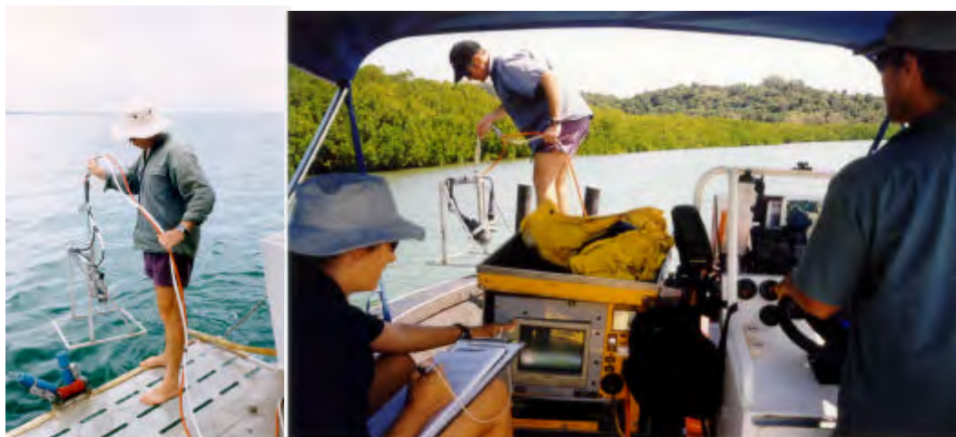
Plate 1. Benthic sampling in coastal areas using vertically deployed video (photo taken in Mourilyan Harbour).
